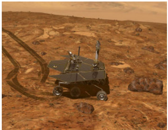
Caption: Opportunity spots a rock with its NavCam that its AEGIS software says meets all the criteria for further investigation.
