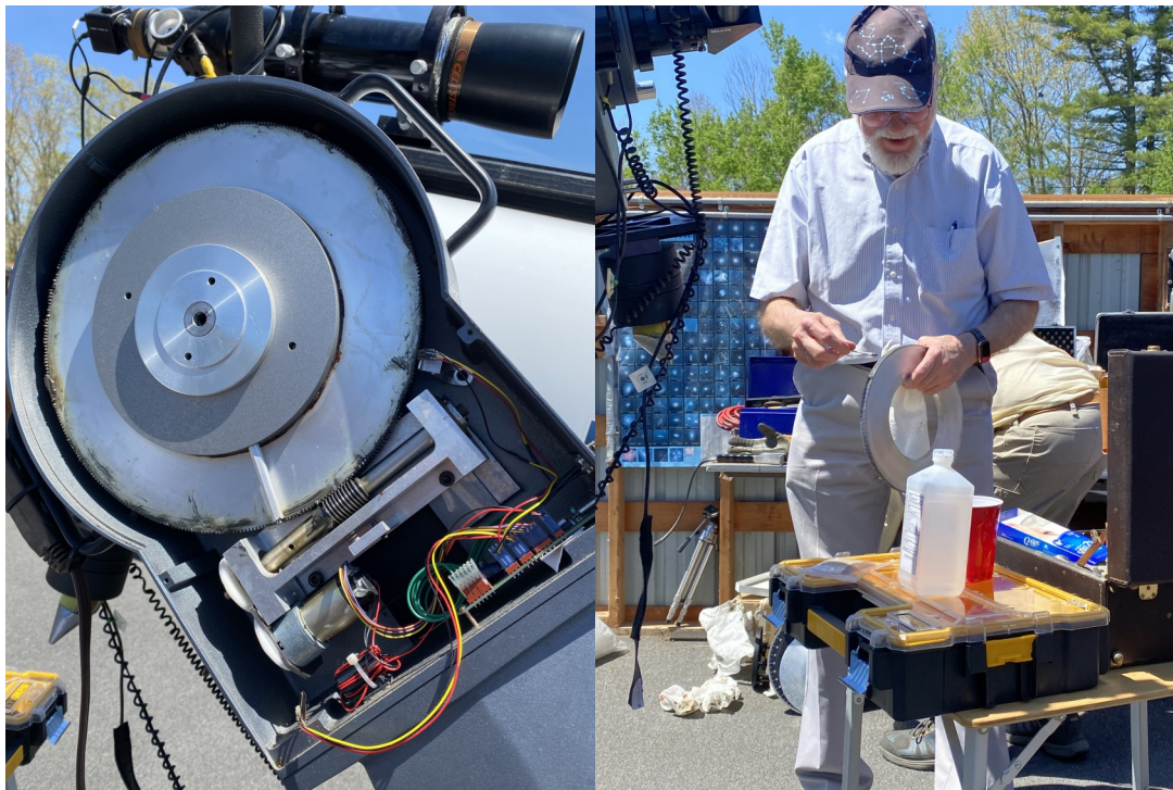
The 16-inch Meade Dec Gear was removed, cleaned and greased.
